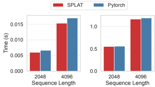
Fig. 11. A comparison of gemma-2 2B’s original implementation (Pytorch) against when its sparse-MHSa mechanism is replaced with SPLAT generated kernels (SPLAT) at varying sequence lengths. Left is a single sparse-MHSa layer and Right is an end-to-end transformer.
